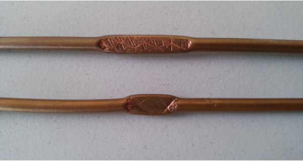
Fig. 2: Partially crushed semi-rigid coaxial cables used for creating the two faulty samples for the experimental validation of the TR-MUSIC approach where the fault's reflection coefficient increases with an increase in the crushed area.
