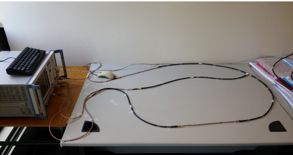
Fig. 3: The experimental setup of the double fault single Y-junction cable network of Fig. 1 (b), which shows the NUT's extremities connected to the vector network analyzer ZVB8 VNA.
