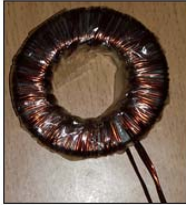
Figure 9. Realized coil of 2,48 mH.
