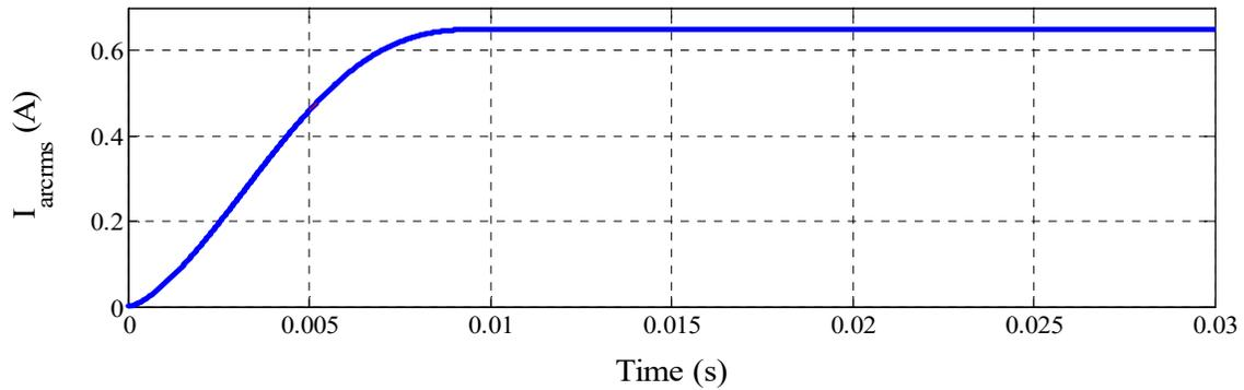
FIGURE 8. Effective arc current in close loop.
