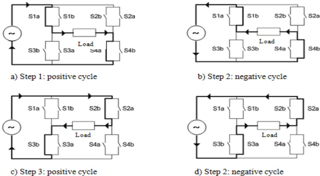
FIGURE 2.The 4 possible operating configurations of the SPMC, [9-11].
