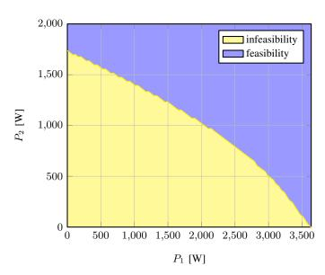
Fig. 6. Feasibility and infeasibility regions of  $R_P(T) > 0$  for the circuit of Fig. 5.
