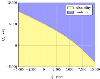
Fig. 7. Feasibility and infeasibility regions of  $R_Q(\bar{T}) > 0$  for the circuit of Fig. 5.
