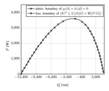
Fig. 4. Boundary of the admissibility set  $S^A$  and feasibility boundary of the inequality  $|K|^2 > 2(|S||G| + \Re\{S^*G\})$ .
