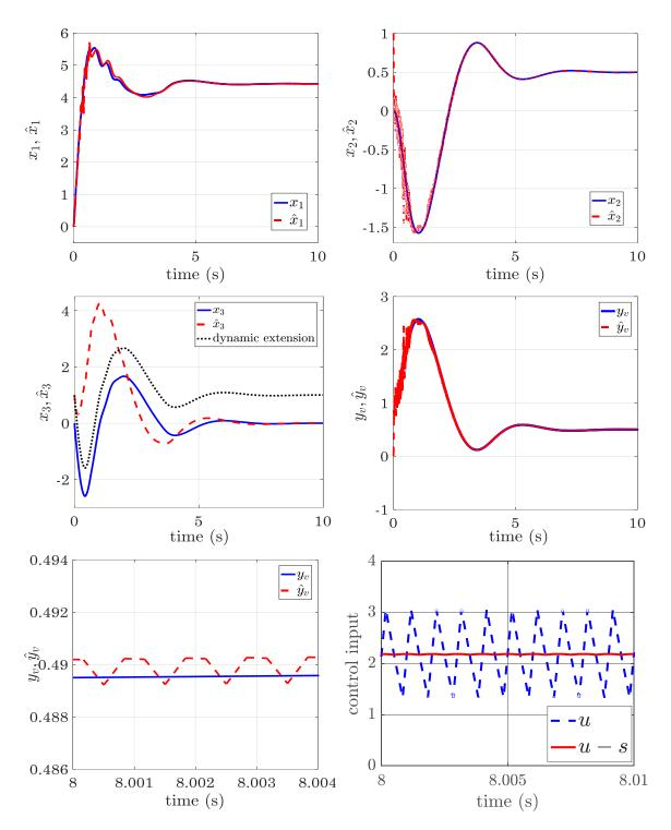
Figure 3: Simulation results of the levitated ball
