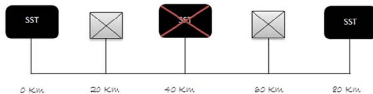
Figure 4: Position of the feeding substations (SST) along the studied line. The substation at 40 km is out of order
