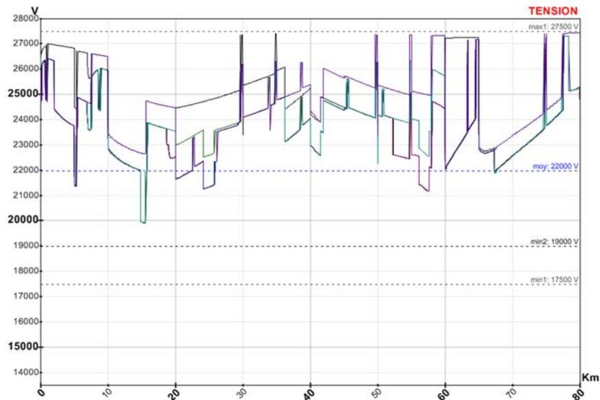
Figure 5: Trains pantographs voltages in the nominal case
