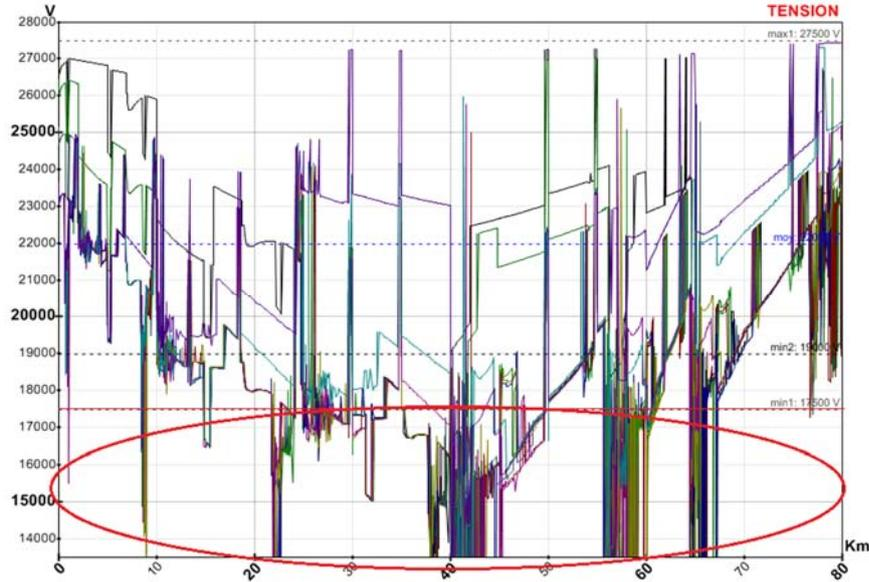
Figure 6: Trains pantographs voltages in the default case
