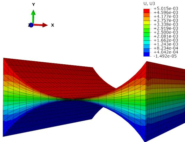
Figure 10: Shearing of the matrix between 2 wires
