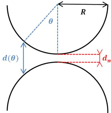
Figure 9: Parameterization of the geometry between two wires
