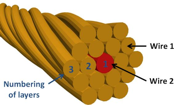
Figure 5: 19-wire cable of length 10 mm
