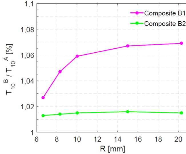
Figure 18: Quantification of the increase of stress due to the presence of infiltrated matrix in composites B1 (high stiffness's  $K$  evaluated in section 3) and B2 (stiffness's  $K$  representative of the real composite)
