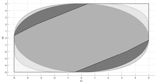
Fig. 4. Polyhedral, Ellipsoidal and pre-specified degree Contractive Sets for Example 2
