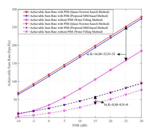
**Fig. 2**. Achievable rate versus SNR.  $R_{min} = \log_2(1 + \frac{\text{SNR}}{2K})$  bps/Hz; a) K = 16, M = 32, N = 32; b) K = 8, M = 8, N = 8.
