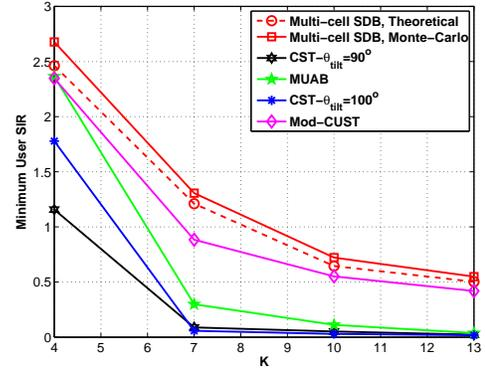
Fig. 3. Performance of SDB in a multi-cell system.
