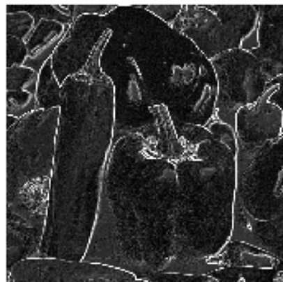
Fig. 8 Gradient computed from the results of Sobel transistor-level simulations of our system on the image of the peppers (see Fig. 2)
