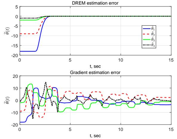
**Fig. 2:** Parameters estimation errors with the gain  $\Gamma_2$ .
