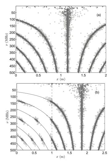
Fig. 4: Local maxima in the pseudo-spectra computed from scattering matrices measured for the two configurations in Fig. 2: (a) single-branch case and (b) single-junction case. Two noise levels are considered, a 15 dB SNR (dark gray dots) and 5 dB SNR (light gray dots), with solid black lines the theoretical results expected from (2).
