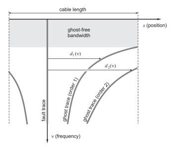
Fig. 1: Typical structure of the pseudo spectrum  $\Phi(x,\nu)$  generated by TR-MUSIC for a cable, as the locus of points over the frequency-position plane where the pseudo-spectrum presents singularities.
