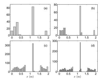
Fig. 6: Number of peaks per bin for the results in Fig. 4(a), for the single-cable case and a 15 dB SNR. The four histograms correspond to  $1/\alpha=5.5$  and 10.5 (left and right columns), for data collected on the frequency ranges 100-150 MHz and 100-300 MHz (top and bottom rows).
