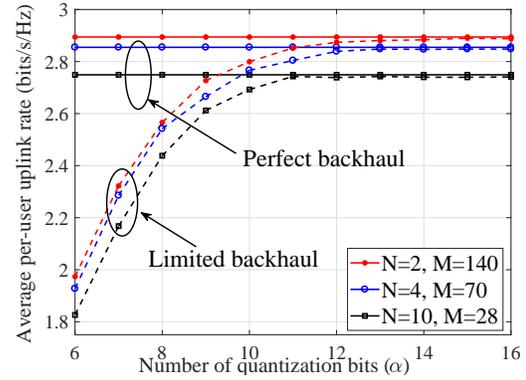
Figure 1. Average per-user uplink rate versus the number of quantization bits,  $\alpha$ , with limited and perfect backhaul link.
