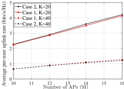
Figure 5. The average per-user uplink rate for cases 1 and 2, with ( $N = 4$ ,  $K = 20$ ,  $\tau = 20$ ,  $\alpha_1 = 9$ ,  $\alpha_2 = 2$ ,  $\omega_g = 3$ ,  $\omega_y = 80$ ,  $\omega_z = 3$ ), and ( $N = 20$ ,  $K = 40$ ,  $\tau = 40$ ,  $\alpha_1 = 8$ ,  $\alpha_2 = 5$ ,  $\omega_g = 3.5$ ,  $\omega_y = 70$ ,  $\omega_z = 3$ ) with  $D = 1$  km and  $\tau_c = 200$ .
