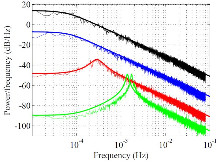
Fig. 6 – Spectra of amplitude ratio fluctuations obtained for different drive levels  $F$ . The thick lines are obtained with the analytical calculations (36-38), the thin lines with transient simulations of (1).
