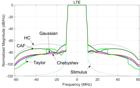
Fig. 4: Test of different windows for CABF
