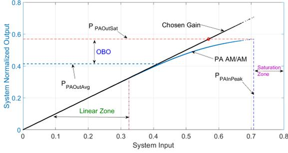
Fig. 2: PA output signal vs PA input signal
