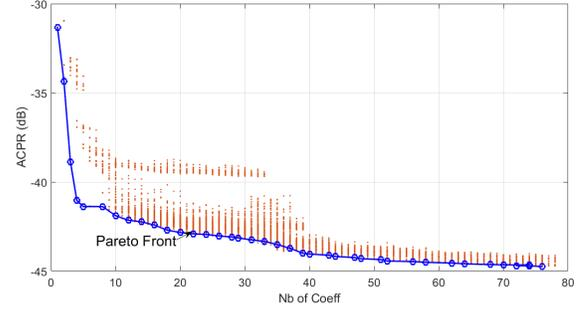
Fig. 2. ACPR vs Number of DPD coefficients
