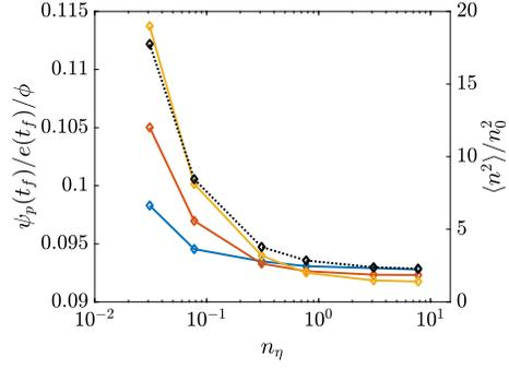
**Figure 13:** Solid lines (—) : fluid-particle coupling energy rate and dotted line (·····) : segregation as a function of particle number density for  $St = 0.4$  at  $t_f = 6$  (respectively left and right axis). Lines blue:  $\phi = 0.1$ , red:  $\phi = 0.2$ , yellow:  $\phi = 0.3$ .
