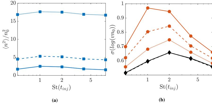
**Figure 5:** Comparison of preferential concentration for one-way coupled simulations. Dotted lines ( $\cdots$ ):  $n_\eta = 0.03$ , dashed lines ( $--$ ):  $n_\eta = 0.15$  and solid lines ( $—$ ):  $n_\eta = 1.5$ . (a) Bin counting method; (b) Standard deviation of normalized Voronoi PDF before (red lines) and after (black lines) depletion in post-processing.
