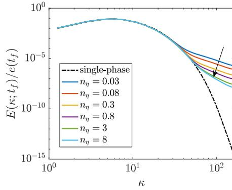
**Figure 14:** Energy spectrum at  $t = 6$  for  $\phi = 0.3$  and  $St = 1.6$ . The arrow shows the increase in the particle number density. The dash-dotted line stands for the single-phase flow spectrum.
