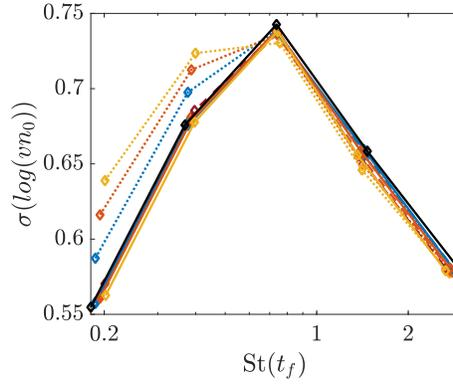
**Figure 19:** Comparison of preferential concentration for all simulations. Lines blue:  $\phi = 0.1$ , red:  $\phi = 0.2$ , yellow:  $\phi = 0.3$ , —:  $n_\eta = 3$ , - - -:  $n_\eta = 0.3$ ,  $\cdots$ :  $n_\eta = 0.03$ . The black dash-dotted line stands for the single-phase flow.
