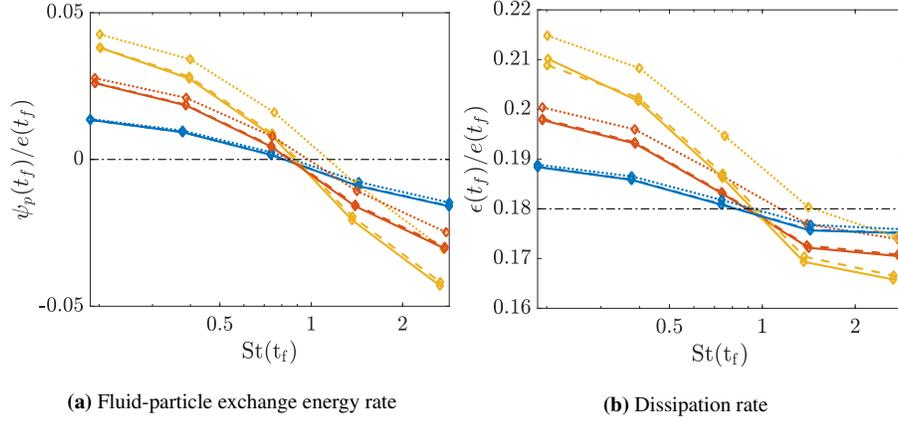
**Figure 9:** (a) Normalized fluid-particle exchange energy rate. (b) Normalized dissipation rate versus Stokes number at time  $t_f = 6$ . Lines blue:  $\phi = 0.1$ , red:  $\phi = 0.2$ , yellow:  $\phi = 0.3$ , —:  $n_\eta = 3$ , ---:  $n_\eta = 0.3$ , .....:  $n_\eta = 0.03$ . The black dash-dotted line stands for the single-phase flow.
