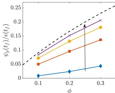
**Figure 11:** Fluid-particle coupling energy rate normalized by dissipation rate as a function of mass loading. The arrow shows the decrease in Stokes number:  $St \in [2, 1, 0.5, 0.15]$ . The dotted line is the asymptotic limit analytically predicted.
