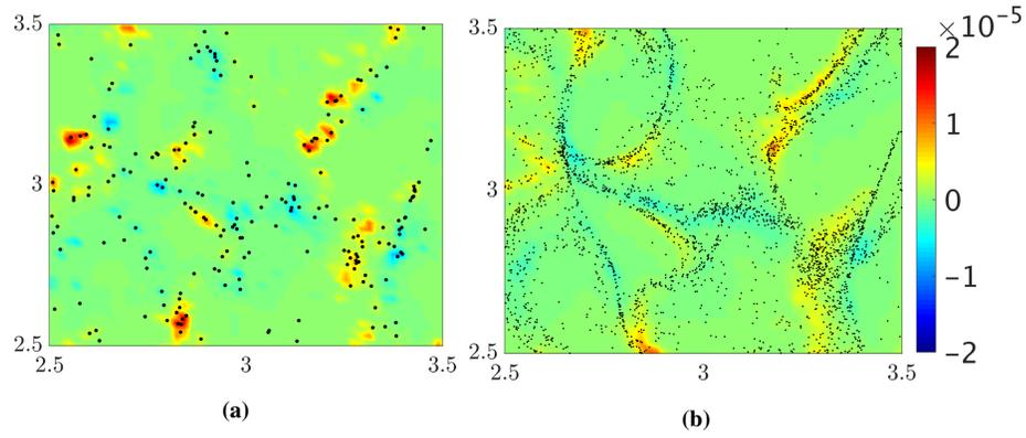
**Figure 17:** Distribution of two-way interaction energy rate  $\tilde{\psi}_p$  at  $t = 6$  superimposed with particles parametrized by  $\phi = 0.001$  and  $St = 1$ . (a)  $n_\eta = 0.12$  ; (b)  $n_\eta = 2$
