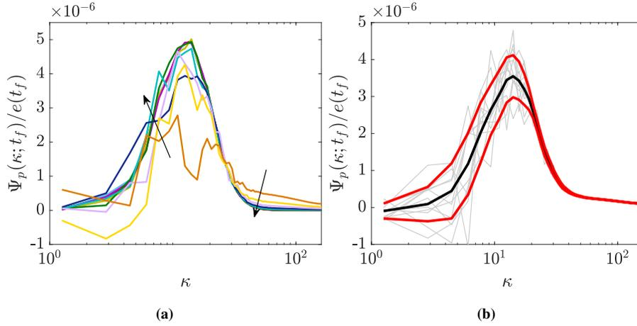
**Figure 20:** (a) Two-way interaction spectra for different particle number densities  $n_\eta = 2.7 \times 2^j$ ,  $j = -15, \dots, 0$ , and fixed  $St = 1$  and  $\phi = 0.001$  (The arrow shows the increase in  $n_\eta$ ). (b) Two-way interaction spectra for 11 realizations of simulation with  $n_\eta = 2.7 \times 2^{-14}$  (grey lines), the mean spectrum (black solid line) and the standard deviation (red solid lines).
