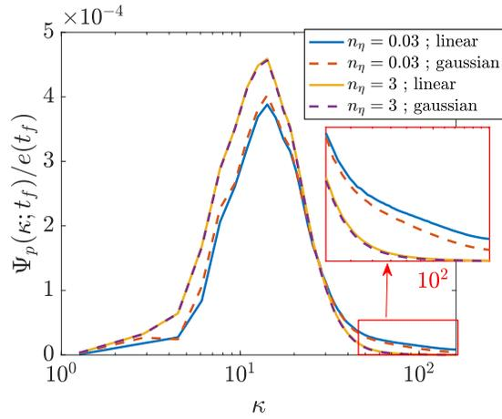
**Figure A.22:** Normalized two-way interaction spectrum with trilinear (solid lines) and gaussian (dashed lines) projection. Two different particle number densities are compared. The inset displays a zoom around the smallest scales.
