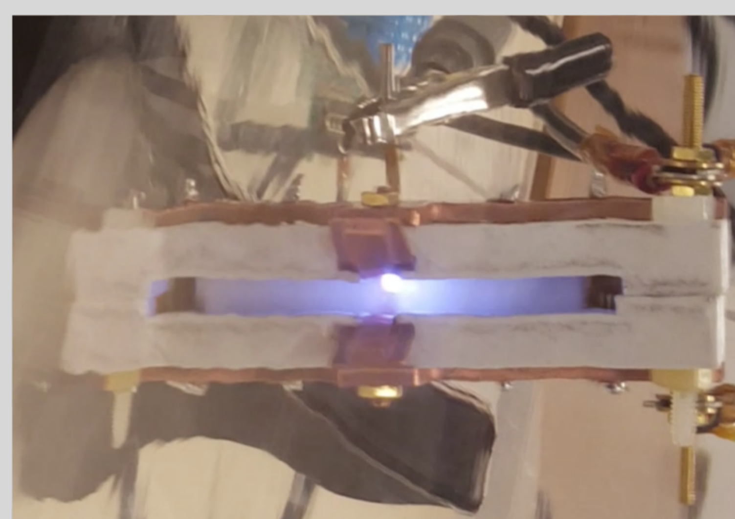
Figure 5: Test performed in vacuum chamber to prove the feasibility of the PPT System at CS 3
