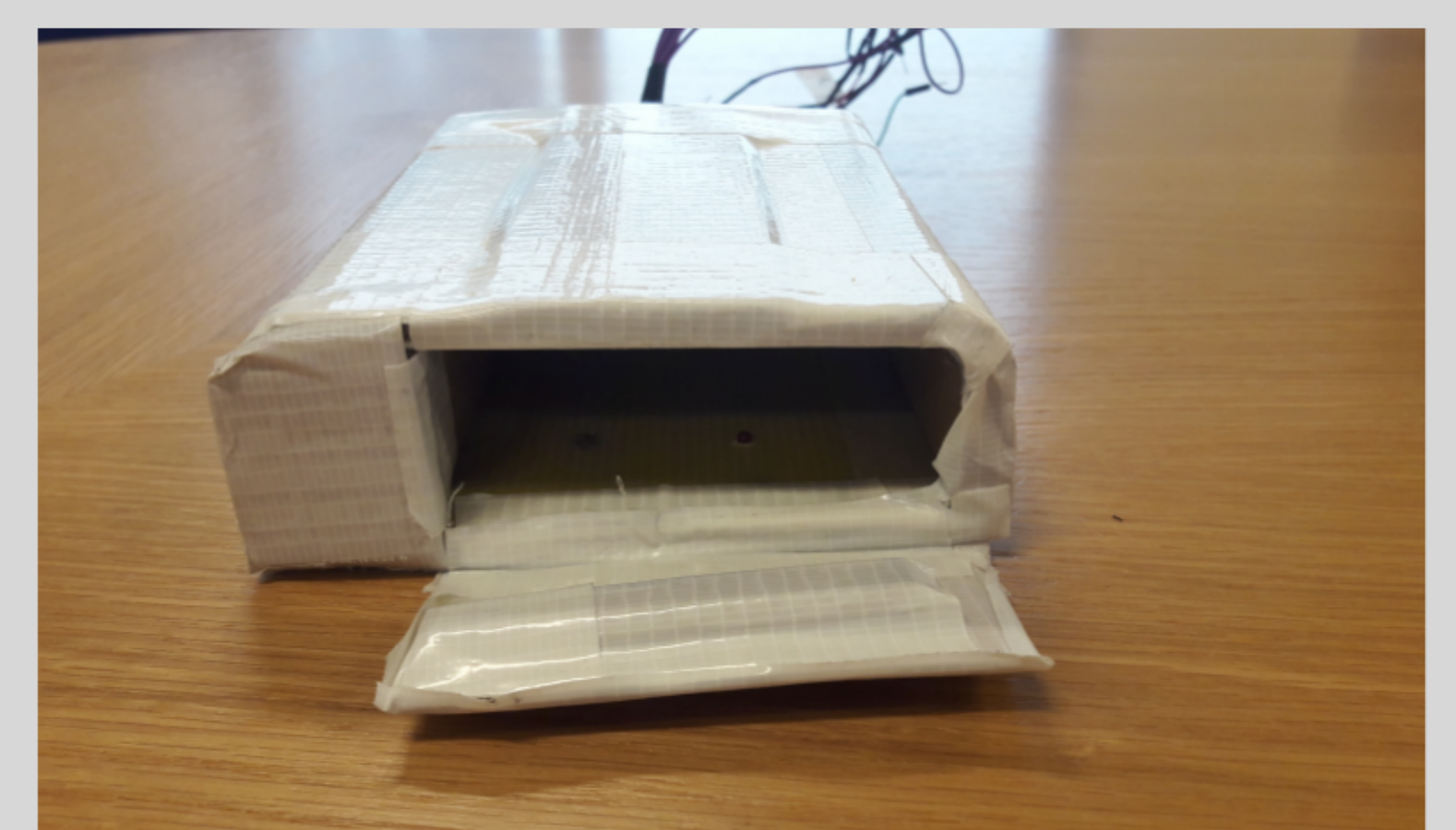
Figure 4: Prototype of a turbidimeter enabling a measurement of the evolution of bacterial concentration in petri dishes
