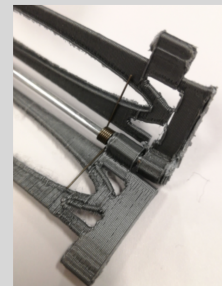
Figure 4: Panels deployment by springs
