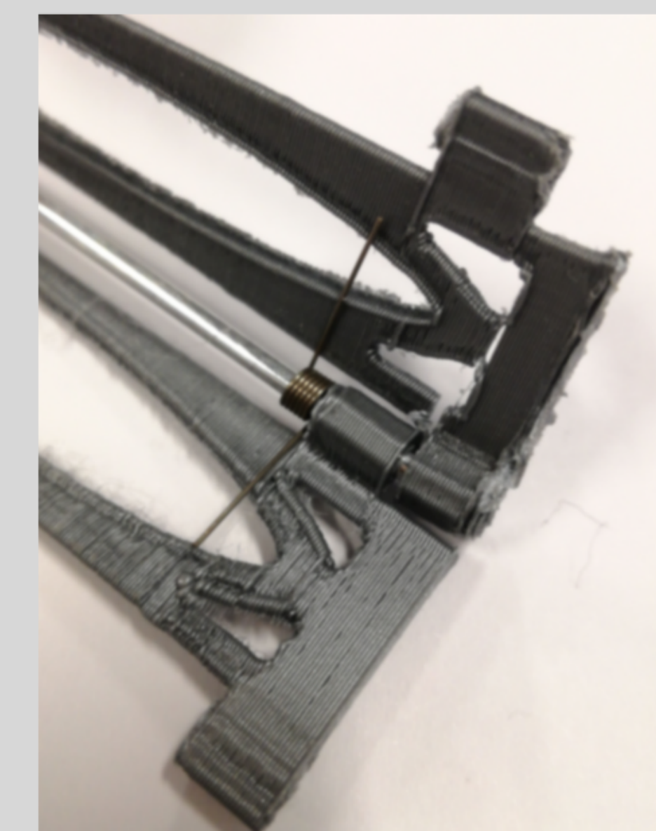
Figure 4: Panels deployment by springs
