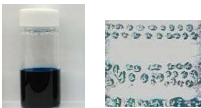
Figure 1. Cu formate AMP (Cuf-AMP) complex dissolved in solvents; visualisation of printed drops incompletely transformed by IPL sintering.
