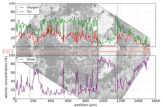
Fig. 11. Atomic concentration of Ag, Sn and O measured by EDS as a function of the position along the red line for an electrode was submitted to 50,000 arcs (300 A rms).
