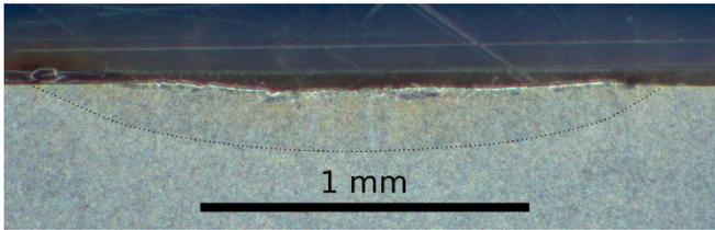
Fig. 8. Cathode microstructure in the cross section along a crater diameter after a single arc (300 A current – case of a flat cathode), observed with an optical microscope.
