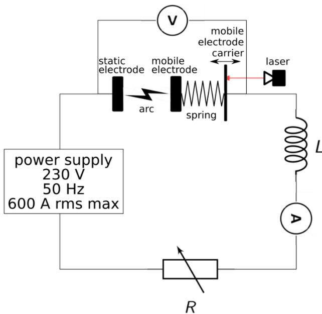
Fig. 1. Electrical circuit diagram; three values of resistances are used to get three current values 150, 300 and 600 A rms; the inductance value is set to get  $\cos(\varphi)=0.35$ ; this machine enables to generate one or several arcs.
