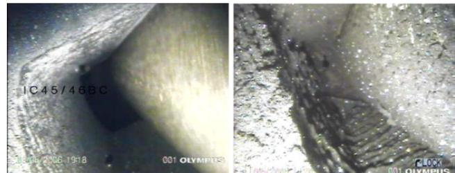
Figure 2. Tube support plate clogging: top view of a clean flow hole on the left side and an entirely blocked flow hole on the right side [9].
