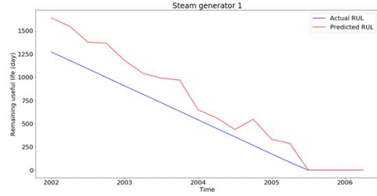
Figure 8. RUL prediction for steam generator No. 1.
