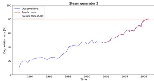
Figure 10. Degradation trajectory prediction for steam generator No. 3.
