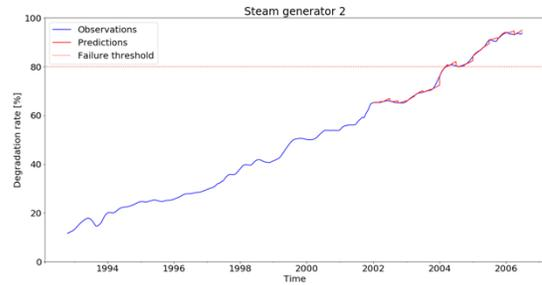
Figure 9. Degradation trajectory prediction for steam generator No. 2.
