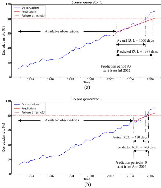
Figure 6. Degradation trajectory prediction for steam generator No. 1: (a) At the 3<sup>rd</sup> prediction period; (b) At the 10<sup>th</sup> prediction period.
