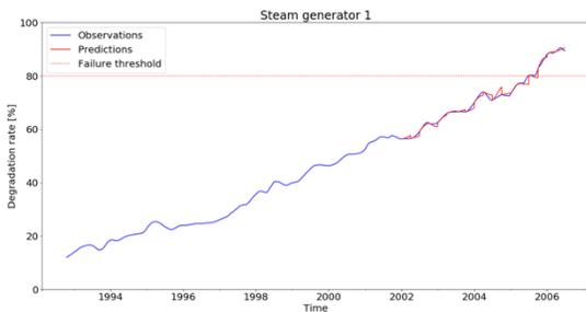
Figure 7. Degradation trajectory prediction for steam generator No. 1.
