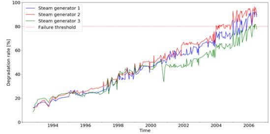
Figure 4. Raw degradation series of steam generator Nos. 1-3.
