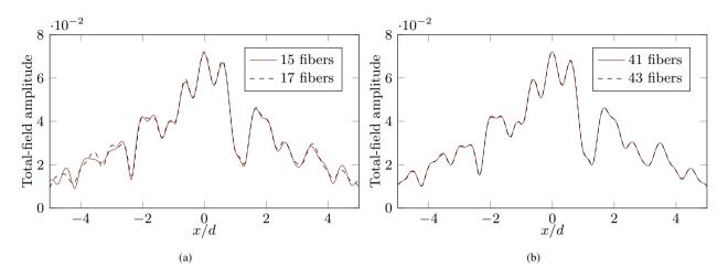
Fig. 9. Amplitude of sampled total fields vs number of fibers in COMSOL,  $\mathbf{r}_s = (0,0)$ ,  $\lambda^{inc} = d$ , z = d, TM polarization.
