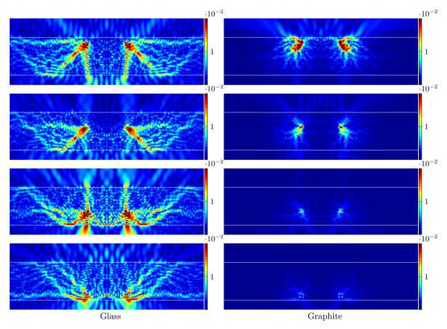
Fig. 14. Maps of anomalous field with the (l, 2)-th and (l, 2)-th fibers missing, l = 1, 2, 3, 4, line source at (0, d),  $\lambda^{inc} = d$ , TM.
