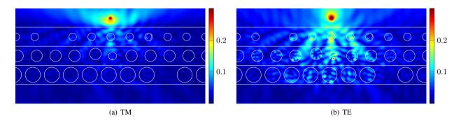
Fig. 11. Amplitude of total (a) electric field and (b) magnetic field with a line-source illumination,  $\mathbf{r}_s = (0, d)$ ,  $\lambda^{inc} = d$ , white lines indicating the laminate structure.
