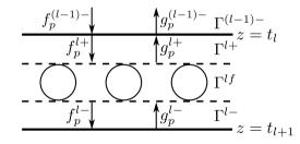
Fig. 2. Coefficients of plane-wave expansions in the *l*-th layer for upgoing and down-going waves.
