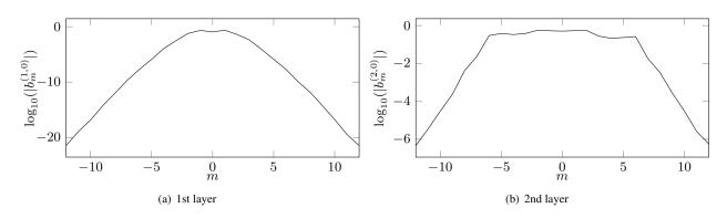
Fig. 7. Line graphs of CWE coefficients  $b_m$ , M = 12, two-layer laminate with the plane-wave illumination,  $\theta^{inc} = \pi/6$ ,  $\lambda^{inc} = d$ .
