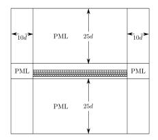
Fig. 8. Geometry of COMSOL module, 43 fibers in each layer of the laminate, fiber radius  $c_1 = 0.2d$ ,  $c_1 = 0.3d$ ,  $c_1 = 0.4d$ .
