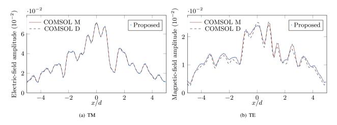
Fig. 10. Validation of the computation of the Green's function by comparisons with COMSOL,  $\mathbf{r}_s = (0,0)$ ,  $\lambda^{inc} = d$ , z = d, "COMSOL D" denoting COMSOL solution with the default mesh settings and "COMSOL M" with manual settings.
