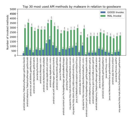
Figure 2. TOP 30 of the highest difference in methods invoked in MAL and GOOD
