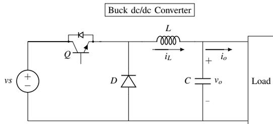
Fig. 1. Topology of the buck DC/DC converter [18].
