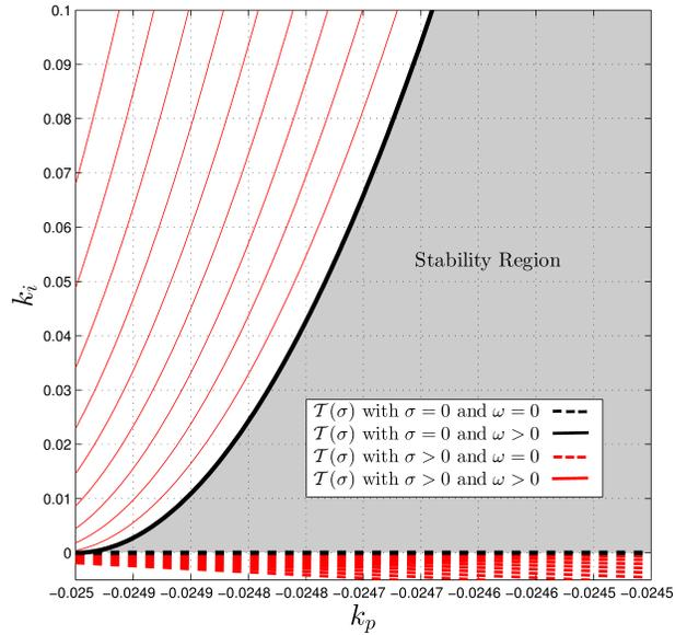
Fig. 2. Stability Analysis in the Parameters Space
