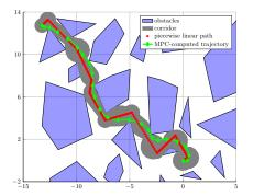
Fig. 5: The shortest path  $Path(x_i, x_f)$  and a feasible trajectory within the corridor.
