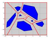
Fig. 1: Space-partitioning using separating hyperplanes.
