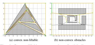
Fig. 6: Convex liftable representation of originally nonliftable obstacles and their associated partition.
