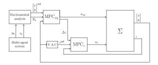
Fig. 5: The control scheme.
