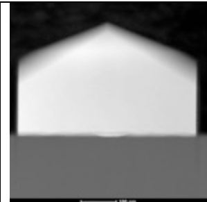
Fig. 3: Dark-field cross-sectional TEM images of the localised GaAs/(111) Si \mu -crystal showing the perfect integration without any antiphase domains nor dislocations nor twins.
