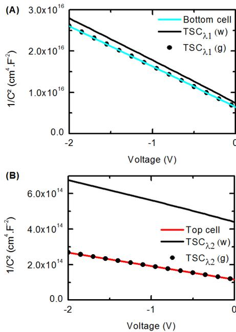
**Figure 5:** Mott-Schottky plots from numerical calculations of  $1/C^2$  values deduced from our simulations of (A) the bottom cell alone in the dark (blue line), the  $\text{TSC}_{\lambda 1}$  when the required conditions are met (black dots) or not (black line) and (B) the top cell alone in the dark (red line), the  $\text{TSC}_{\lambda 2}$  when the required conditions are met (black dots) or not (black line).
