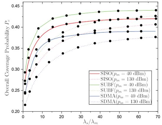
Fig. 5. Overall coverage probability of a MU-MIMO HetNet for varying transmission strategies versus the relative density  $\lambda_s/\lambda_m$  for both noncooperative and cooperative scenarios, where  $\lambda_k = 40\lambda_s$ ,  $p_s = 35 \text{ dBm}$ ,  $M_m = \Psi_m = 1$  and  $M_s = \Psi_s = 1$  (SISO),  $M_m = 8$ ,  $\Psi_m = 1$ ,  $M_s = 4$ ,  $\Psi_s = 1$  (SUBF),  $M_m = \Psi_m = 8$  and  $M_s = \Psi_s = 8$  (SDMA).
