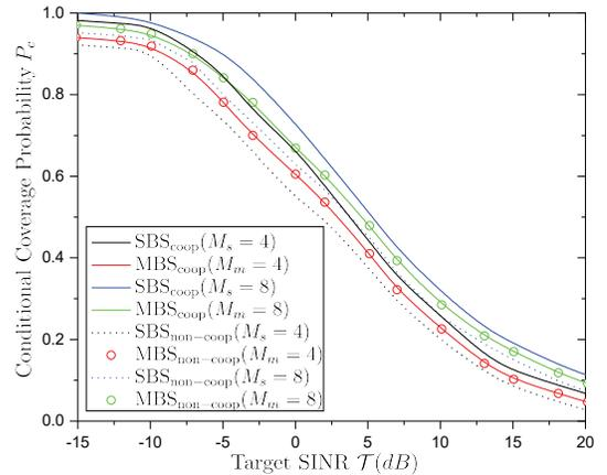
Fig. 3. Coverage probabilities of a MU-MIMO HetNet for varying number of BSs antennas versus the target SINR  $\mathcal{T}$  for both noncooperative and cooperative scenarios, where  $\lambda_m = 0.01 \text{ m}^{-2}$ ,  $\lambda_s = 0.04 \text{ m}^{-2}$ ,  $\lambda_k = 40\lambda_s$ ,  $p_m = 45 \text{ dBm}$ ,  $p_s = 35 \text{ dBm}$ .
