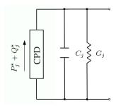
(a) Equivalent circuit scheme for PQ units.
