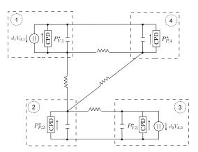
Fig. 2: Four-terminal hvdc transmission system.
