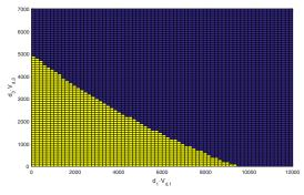
Fig. 3: Feasibility regions of the LMI (III.3) on the plane  $(d_1, d_3)$  of droop control parameters.
