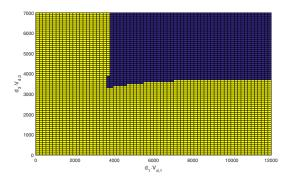
Fig. 4: Feasibility regions of the LMI (IV.3) on the plane  $(d_1, d_3)$  of droop control parameters.
