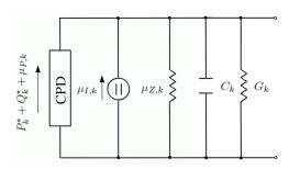
(b) Equivalent circuit scheme for voltage-controlled units
