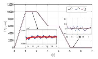
Figure 9: The rotor speed estimation with unknown  $T_L$ .
