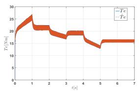
Figure 8: The electromagnetic torque estimation.
