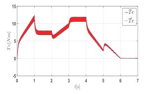
Figure 12: The torque estimation with unknown  $T_L$ .
