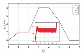
Figure 13: The load torque estimation  $T_L$ .
