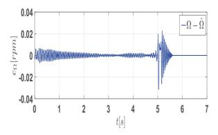
Figure 6: The estimation error of the speed  $(e_{\Omega})$ .
