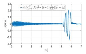
Figure 11: The sliding surface (S) with unknown  $T_L$ .
