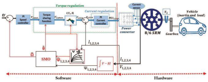
Figure 2: Implementation of the Sliding Mode Observer in the vehicle drivetrain.
