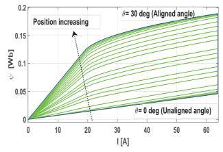
Figure 1: Flux-linkage of the SRM.
