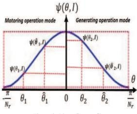
Figure 3: Phase flux profile.
