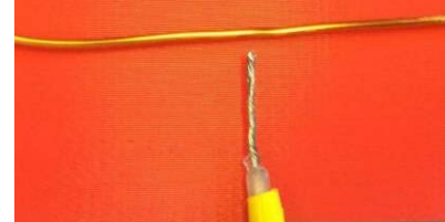
Fig. 8. Coaxial cable sensor
