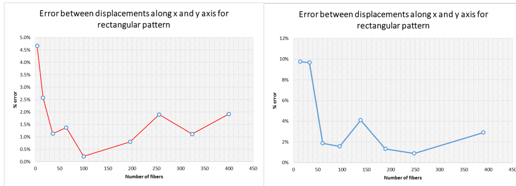
Figure 4: Difference between transversal displacements on opposite vertical faces of the FEM models shown in Figure 3. A small error on the displacements indicates that the assumption of transverse isotropy is valid, and that the FEM domain is a REV.
