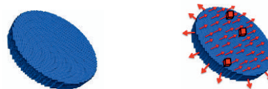
Figure 2. Overview of the sample modeled with square mesh (30000 elements) - Initial state corresponds to the sample.
