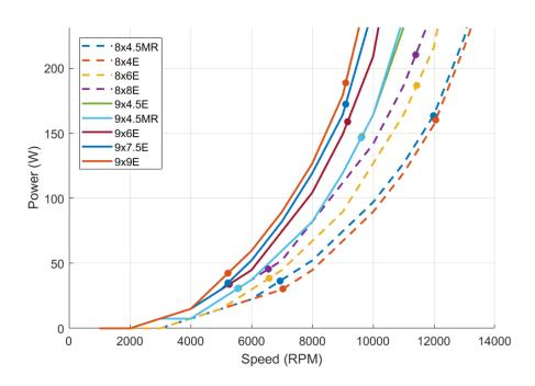
Figure 10: Comparison of power-speed characteristics of 8 and 9 inch propellers.
