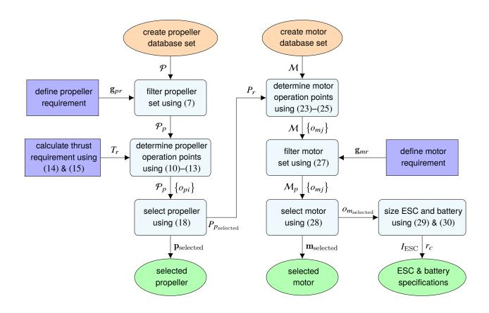
Figure 6: Actuating system sizing methodology information flow diagram.
