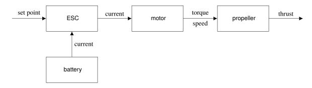
Figure 2: Multirotor propulsion chain diagram.
