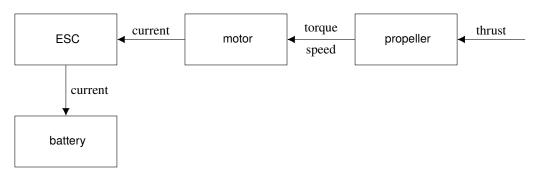
Figure 3: Inverted multirotor propulsion chain diagram.
