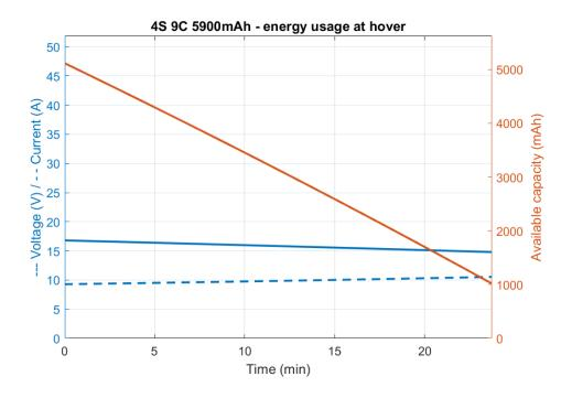
Figure 8: Example battery behaviour during hover.
