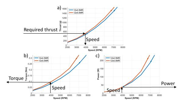
Figure 5: Example of obtaining a propeller operating point based on required thrust. *a*) Obtaining speed from required thrust. *b*) Obtaining torque from speed calculated in *a*). *c*) Obtaining power from speed calculated in *a*).
