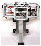
FIGURE 1. We are developing a biped that uses four control moment gyroscopes (highlited in red) as an auxiliary stabilization system.
