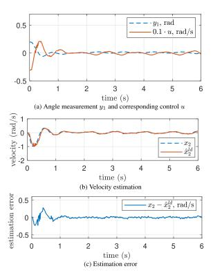
FIGURE 5. Closed-loop stabilization using observer (9).
