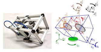
**FIGURE 2.** Left: inverted pendulum hardware that we study in this paper. The pendulum consists of six bodies: body A (the thrust bearing), body B (the frame), bodies  $C^1$  and  $C^2$  (the single-axis gimbals), and, finally, bodies  $D^1$  and  $D^2$  (the flywheels). Right: corresponding notations. This configuration corresponds to  $q_b = -\pi/4$  and  $q_c^1 = q_c^2 = \pi/2$ .
