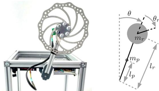
FIGURE 2. 1D pendulum hardware and corresponding notation.
