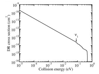
**Figure 4.** DR cross-section as a function of the collision energy. For energies above 0.1 eV, several vibrationally excited channels are open. As a result, the DR cross-section decreases in a stepwise manner.
