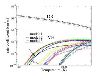
**Figure 6.** DR and VE rate coefficients obtained within three different scattering models – see text. The Model 1 is that described in Section 2. In the Model 2, the basis to represent the electronic wave functions is reduced. In the Model 3, the orbital space in the configuration interaction calculation was reduced with respect to that used in the Model 1. The differences between results obtained in the three models are about 20 per cent.
