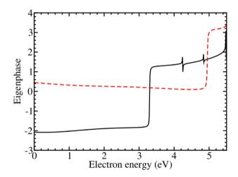
**Figure 3.** Energy-dependence of eigenphases sum of the  $A^{'}$  (solid line) and  $A^{''}$  (dashed line) irreducible representations for the NH<sub>2</sub>CHOH<sup>+</sup> + e<sup>-</sup> scattering.
