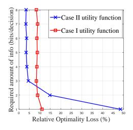
Fig. 3. The impact of  $B_2$  on the preceding observation is assessed. Here, with  $B_2 = 6$  bits/decision, the curves are much steeper, indicating that the choice of the number of feedback rate is more critical in this regime as soon as small optimality losses are desired.
