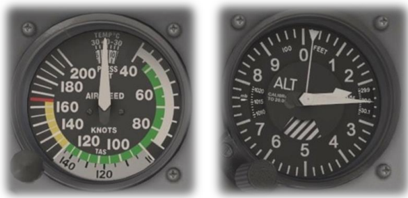
Figure 2: Airspeed indicator and altimeter (courtesy of Laminar Research)
