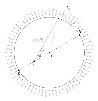
Figure 13: Light attenuation in a cylindrical geometry
