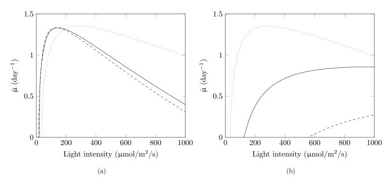
Figure 9: Population level growth rate at versus incident light intensity, at an OD of 0.2 (a) and 1.0 (b). Solid line: taking cells motion into account, dashed line: Han's model applied locally without taking microalgae motion into account, doted line: Han's model applied only using incident light intensity and without taking microalgae motion into account
