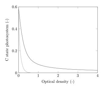
Figure 11: Fraction of the photodamaged photosystems at the population level. Light intensity: 2 000  $\mu$ molPhoton/m<sup>2</sup>/s. Black line: stirrer set at 100 rpm. Gray line: stirrer set at 50 rpm
