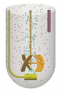
Figure 3: Visualization of the photobioreactor. Aeration: 0.1 vvm, stirring: 100 rpm. Lagrangian tracers: 10 000, only 100 represented (randomly drawn). Time: 1 minute. Color legend: blue - bubbles, red - tracers, orange - stirrer, yellow - sparger, purple - pH probe
