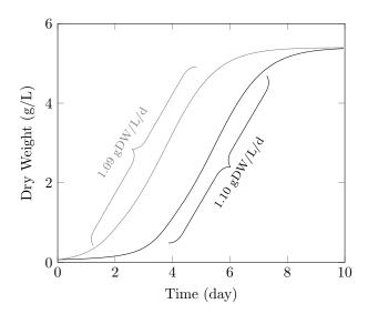
Figure 10: Predicted microalgal density inside of the reactor. Black line: two steps lighting strategy - 500  $\mu$ molPhoton/m<sup>2</sup>/s until an optical density of 1.0 is reached, 2 000 afterwards -. Gray line: optimal lighting strategy. Initial optical density: 0.05 / Initial dry weight: 0.1 g/L
