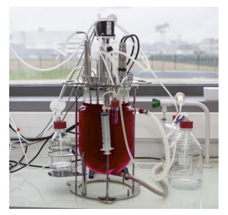
Figure 1: Picture of the actual photobioreactor to be investigated
