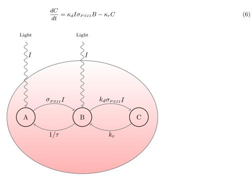
Figure 5: Schematic representation of Han's model. Red ellipse: cell. Circle: photosystem. A: open state, B: processing state, C: photodamaged state [39]
