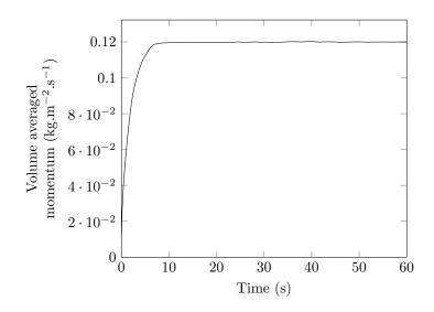
Figure 12: Volume averaged momentum. Aeration: 0.1 vvm, stirring: 100 rpm
