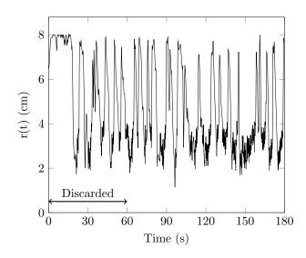
Figure 4: Radial position of a randomly drawn tracer over the first 3 minutes of computation with a stirrer set at 100 rpm
