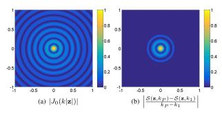
**FIGURE 5.** Two-dimensional plots of  $|J_0(k|\mathbf{z}|)|$  for f=1 GHz and  $|(\mathcal{S}(\mathbf{z},k_P)-\mathcal{S}(\mathbf{z},k_1))|/(k_P-k_1)|$  for  $f_1=700$  MHz and  $f_P=1.3$  GHz.
