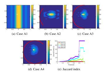
**FIGURE 6.** (Example 5) Maps of  $\mathfrak{F}_{MDSM}(z)$  and Jaccard index with  $f = \{700 \text{ MHz}, 800 \text{ GHz}, \cdots, 1.3 \text{ GHz}\}$ , where the red points represent  $\theta_B$ .
