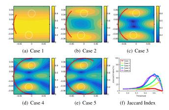
**FIGURE 4.** (Example 4) Maps of  $\mathfrak{F}_{DSM}(z)$  and Jaccard index with f = 4 GHz, where the red points represent  $\theta_B$ .
