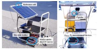
Fig. 2. Experimental setup of outdoor short-time test
