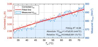
Fig. 3. Indoor test result with average  $G_{POA}$  at 883  $W/m^2$
