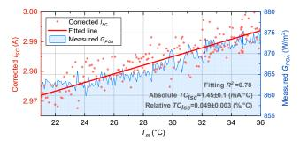
Fig. 5. Outdoor test result with average  $G_{POA}$  at 868  $W/m^2$
