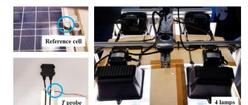
Fig. 1. Experimental setup of indoor controlled -irradiance test
