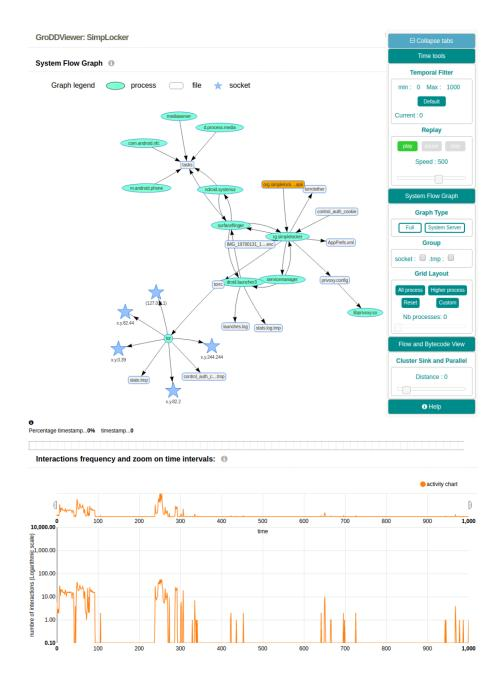
**Fig. 1.** Overview of GroDDViewer (part 1): System Flow Graph (upper part) – Interactions frequency (bottom part) – Malware investigated: Simplelocker (cf. Section 5)
