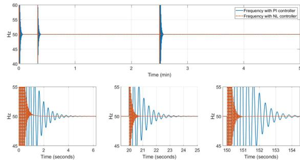
Fig. 7. The frequency variation in the AC side.
