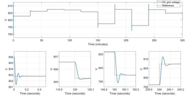
Fig. 13. The DC bus voltage dynamic with CPL.
