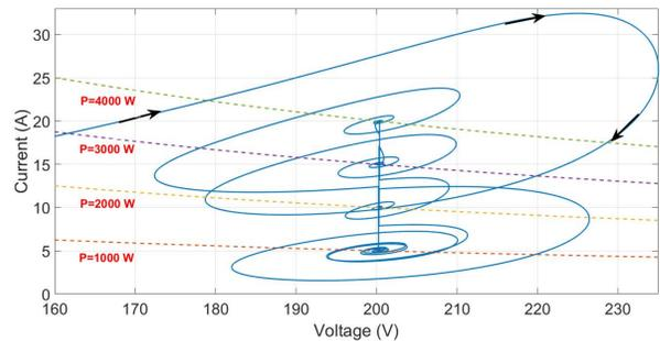
Fig. 15. The V-I trajectories in the CPL case.
