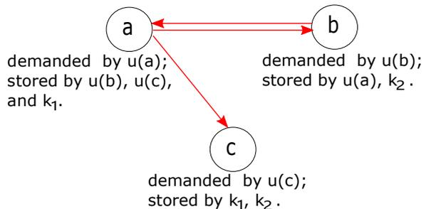
Fig. 3: Directed graph of the two-sender ( $k_1$  and  $k_2$ ) distributed index problem in Proposition 1. A direct edge from node  $a$  to node  $b$ , means that receiver  $u(b)$  demanding message  $b$  stores message  $a$  demanded by receiver  $u(a)$ .
